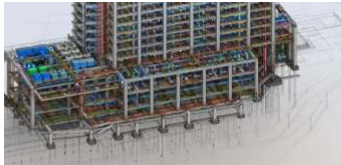
Gambar 4. Model BIM MEP
