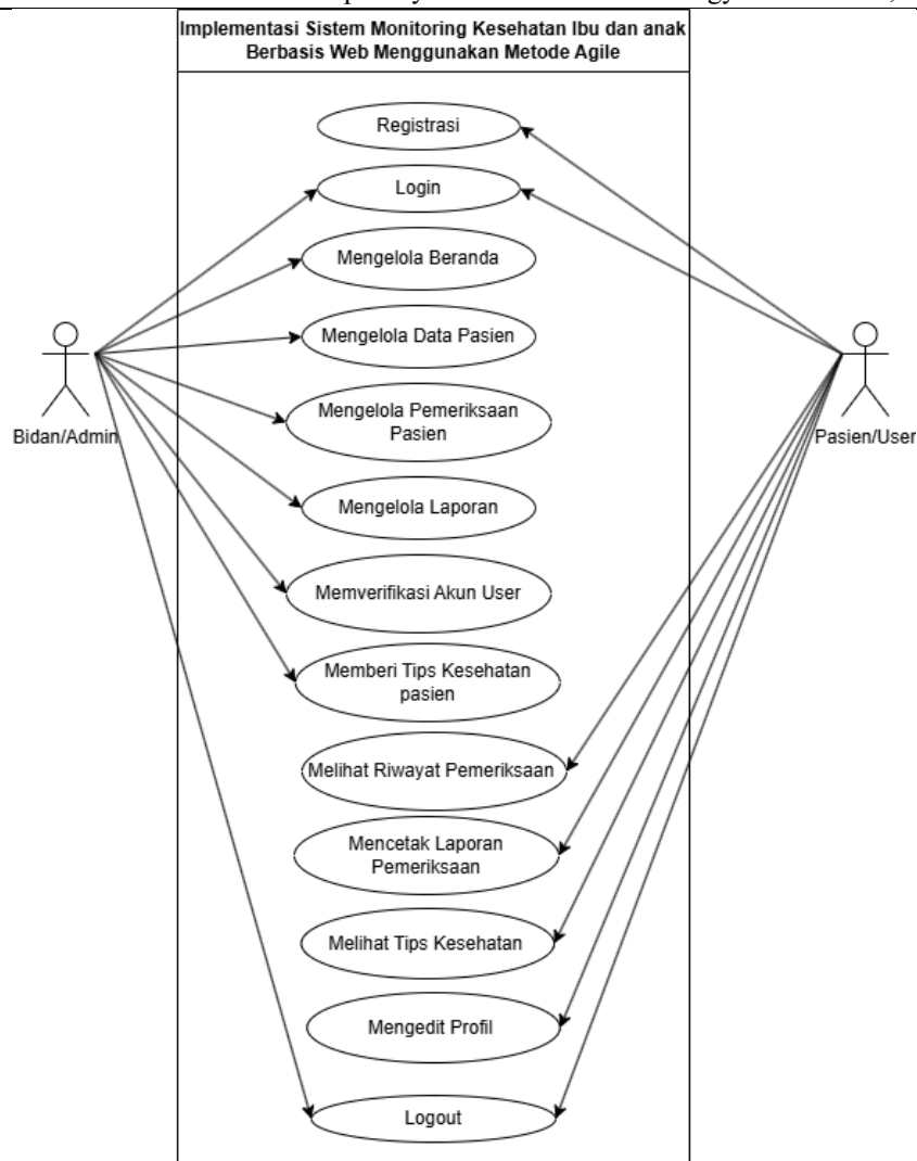
Gambar 2 Use Case Diagram
