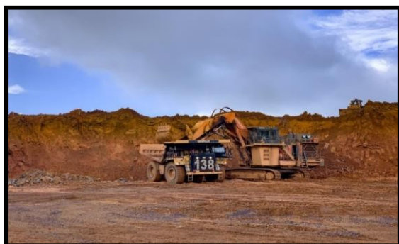
Gambar 5. Proses kegiatan pengisian material (loading)
