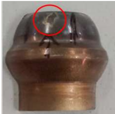
Figure 3. NG black dot part GDI PT UII (Source: NG In process PT UII,2025).
