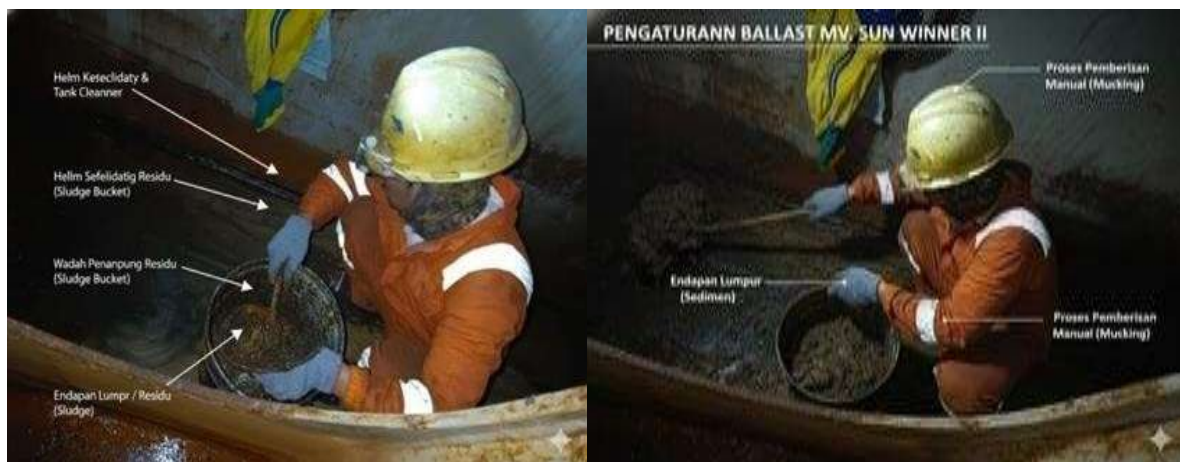
Picture 6. Sludge Removal
