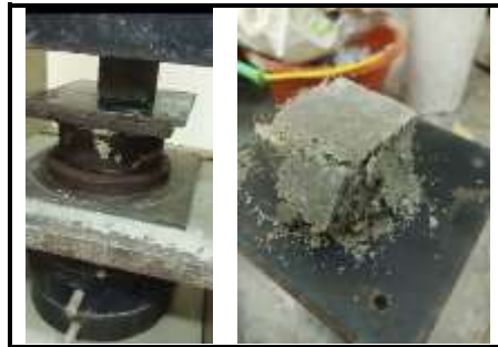
Figure 6. Documentation of Compressive Strength Testing
