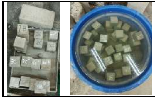
Figure 4. Documentation of Water Absorption Testing
