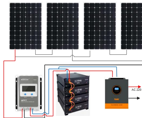
Gambar 7. Wiring PLTS 3000 watt
