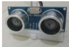
Figure 6 HC-SR04 Ultrasonic Sensor Used for Feed Stock Level Measurement
