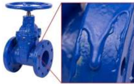
Gambar 2.5 Defect Uneven coating
