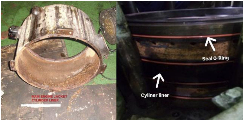
Gambar 2. Main engine jacket cylinder liner
