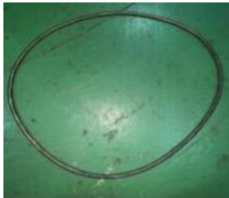
Gambar 3. O-Ring Jacket cooling cylinder liner
